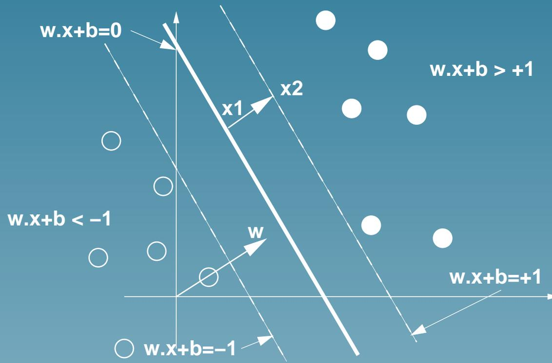
**The width of the tube is  $1/||\vec{w}||$**
